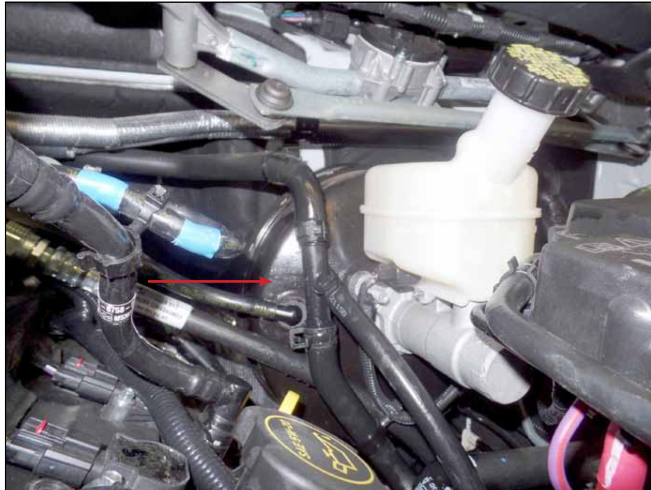
Coolant Y facing down towards the engine compartment.
